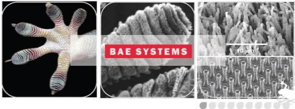
The development of Gecko tape was inspired by the gecko's ability to climb vertical surfaces and upside down and easily peel their feet off the surface again. This ability is due to Van der Waal's forces, which are weak intermolecular attractive forces.
